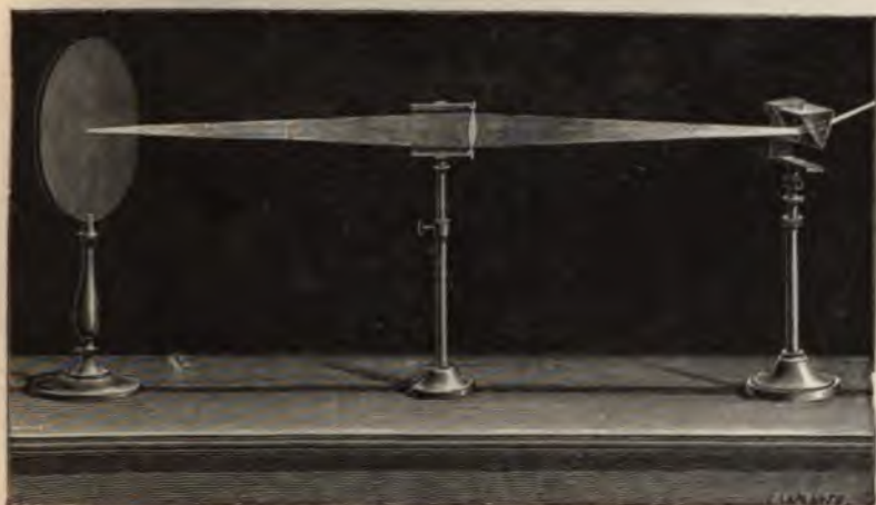
FIG. 41.—Recomposition of white light by means of a lens.
